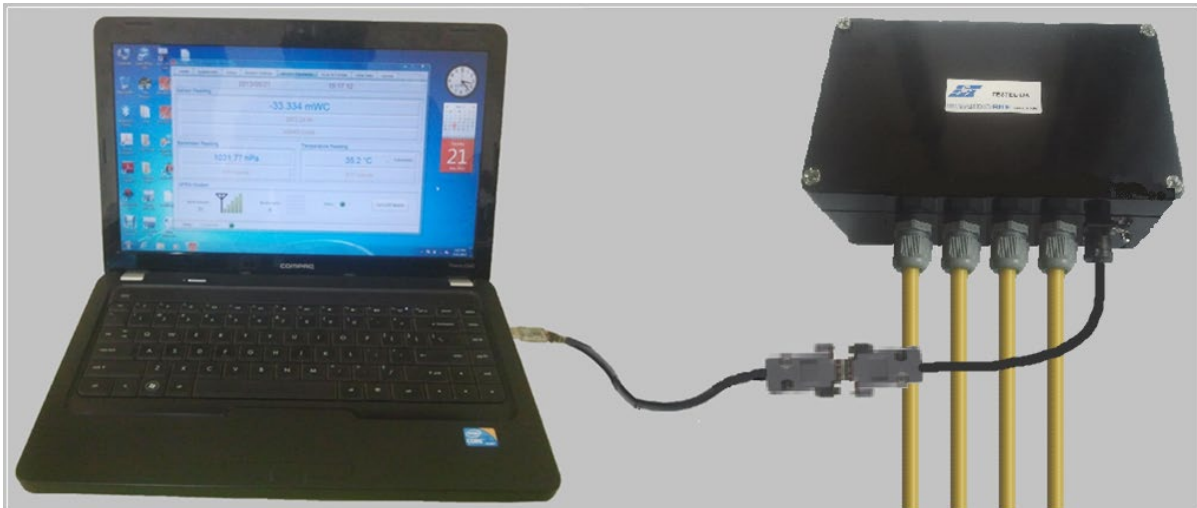
Figure 2-3 : Connecting data logger using interface cable
