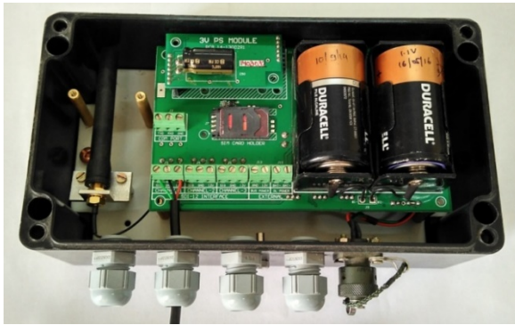
Figure 10-1: Battery replacement for Alkaline battery option
