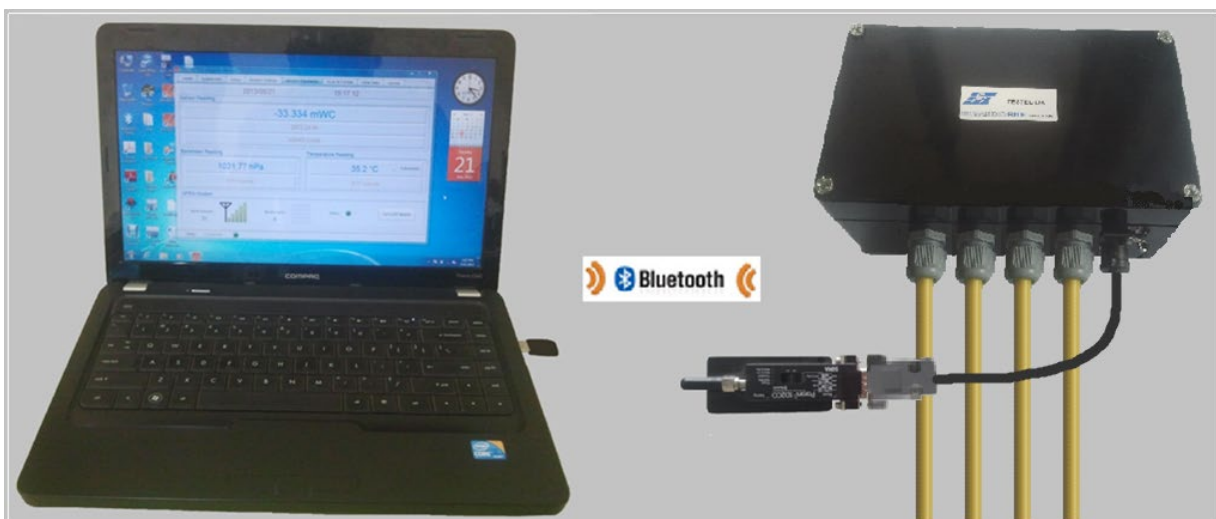
Figure 6-7: Connecting Datalogger with Laptop using Bluetooth Modem
