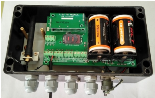
Figure 10-2: Battery replacement for Li battery option
