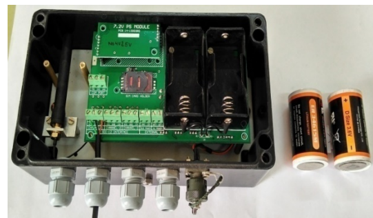
Figure 10-2: Battery replacement for Li battery option
