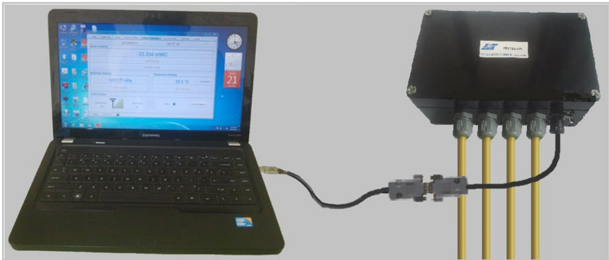
Figure 6-3: Datalogger connection using communication cable
