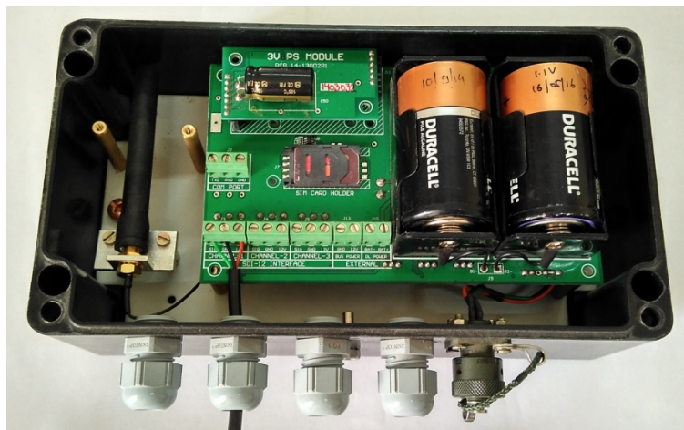
Figure 4-1 Datalogger powered with 2 x 1.5 V Alkaline Batteries
