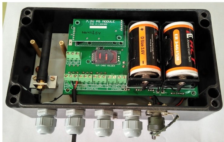
Figure 4-2 Datalogger powered with 2 x 3.6 V Lithium Batteries
